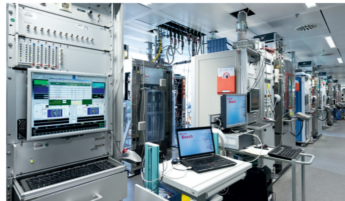
Continuous operation test benches at Bosch's laboratory: Continuous quality testing ensures that ENV6 reliably supports high performance and service life of modern braking systems.
