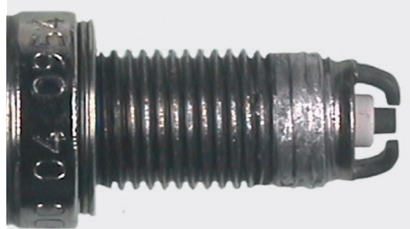
Molten aluminum of the cylinder head in the steel thread of the spark plug
