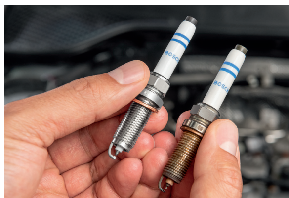
Comparison of a used and a new spark plug
