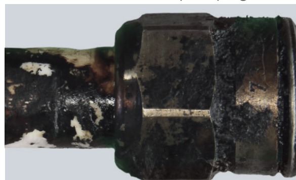
Dirt on the spark plug
