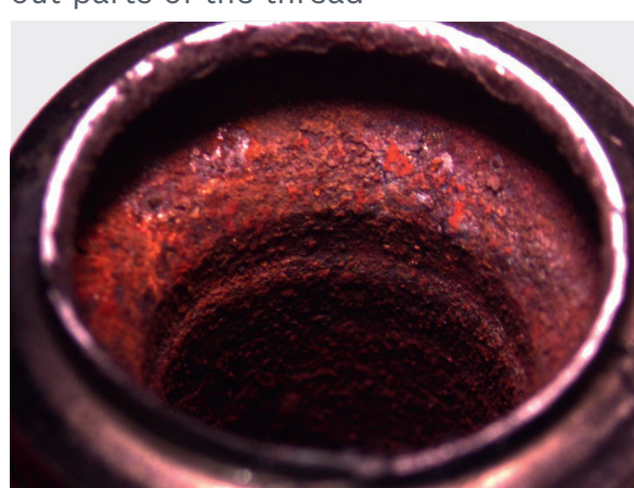
Corrosion inside the spark plug, caused by lack of gas-tightness.
