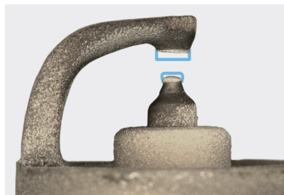
Electrode gap in new and used condition (graphic illustration)
