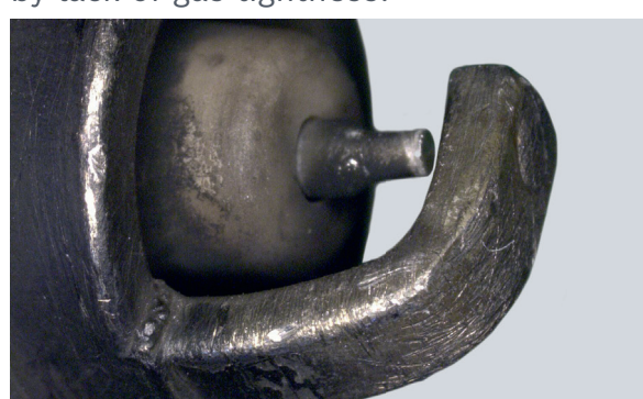
Electrodes damaged by cleaning with a wire brush
