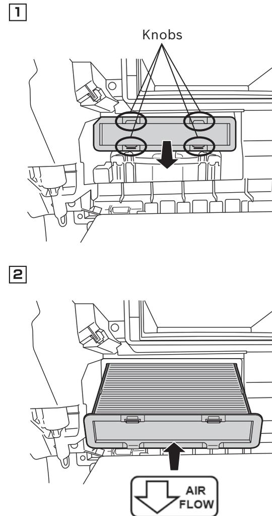
1. Pinch the knobs on the filter cover and pull the filter cover towards yourself.
