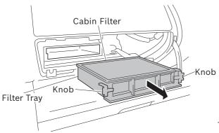
1. Hold the left and right knobs of the filter tray, and pull it out from the front.
