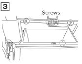
Remove the screws (6 places) and pull the panel towards you to remove it.
