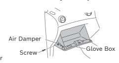
Open the glove box and remove the air damper and screw. Press inwards to remove the
