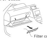
Open the glove box and remove the cover located at the back of the glove box. Do not remove glove box.
