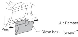
Open the glove box and press from both sides to remove the pins (2 places). Press inwards to remove the glove box.
