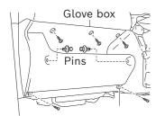
Open the glove box and remove the screws (5 places) and pins (2 places).
