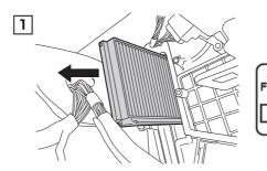
1. Pull out the upper filter, then raise and pull out the lower filter
