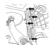
1. Remove the screws (4 places) and remove the filter cover
