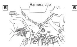
1. Remove the harness clip (1 place) on the back of the fuse box
