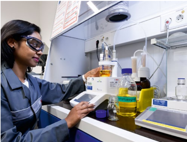
Bosch ENV6 test results at the laboratory: at the Bosch development center, the brake fluid is subjected to chemical tests.
