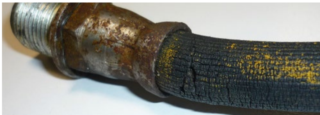
Corroded brake hose
