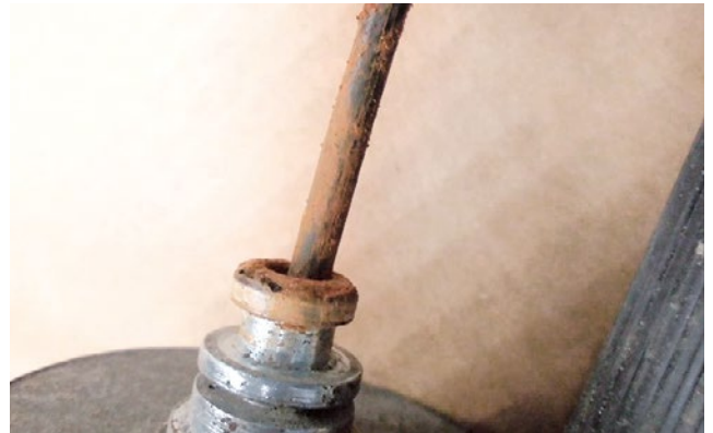
Corroded and tight brake cable
