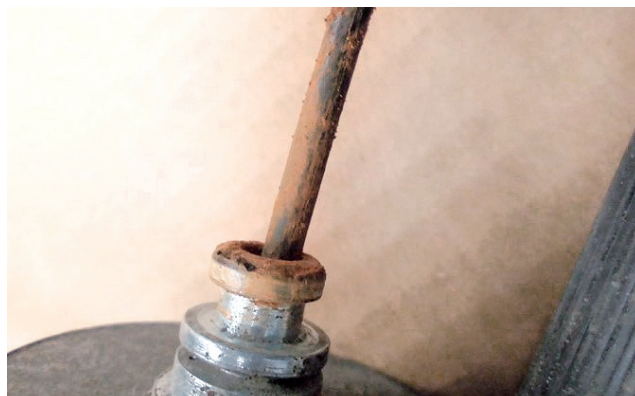
Corroded and tight brake cable
