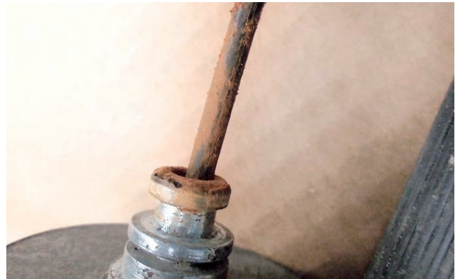
Corroded and tight brake cable
