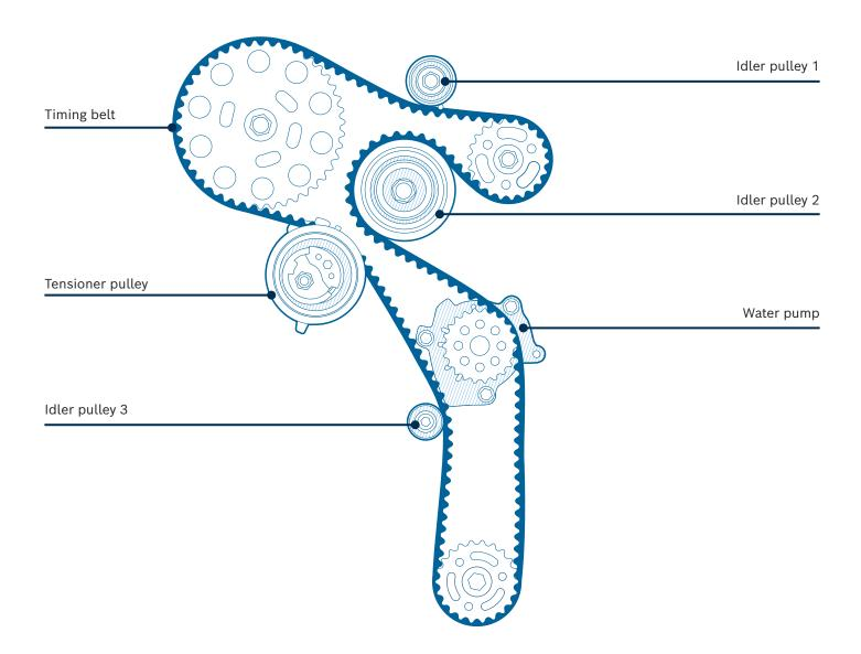
Interaction of all components in the system Timing belts, timing belt kits and water pump kits – complete with all components – ensure a powerful and synchronous long-term power transmission.
