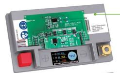
Battery lid with voltage tester and balancer (passive balancing of battery cells)
