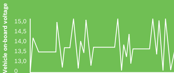
Battery straining in case of start/stop with regenerative braking
