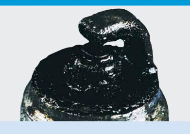
Insulator nose, electrodes and spark-plug shell covered with shiny soot or carbon deposits.
