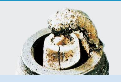
Center electrode melted, ground electrode also severely corroded.
