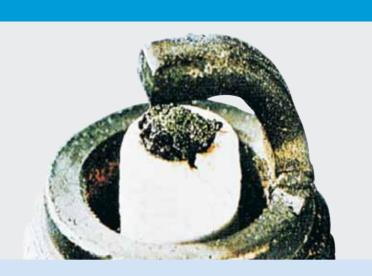
Center electrode partially melted, blistered, spongy, soft insulator nose tip.
