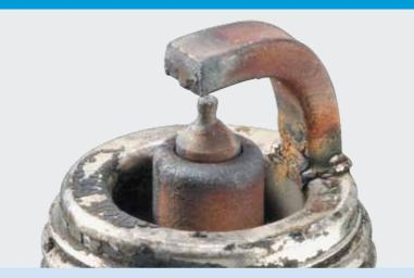
Insulator nose, electrodes and part of the spark plug housing coated with red-orange adherent deposits.
