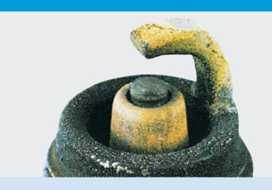
High material abrasion at the center electrode due to wear
