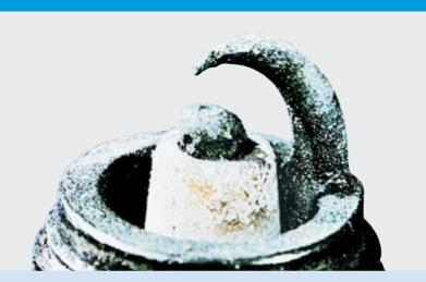
High material abrasion at the ground electrode due to wear
