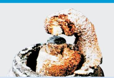
Thick ash coating from oil and fuel additives on insulator nose, in scavenging area (annular orifice) and on ground electrode. Loose to cinder-like structure.
