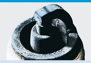
Insulator nose, electrodes and spark-plug shell covered with velvet-like dull black soot deposits.
