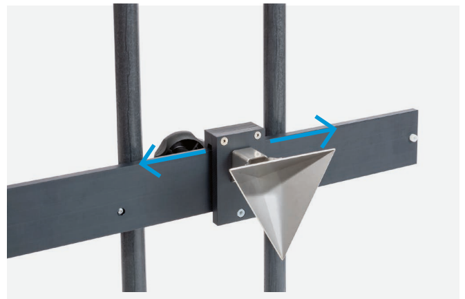
Target with transverse displacement: accurate offset scale gives guidance
