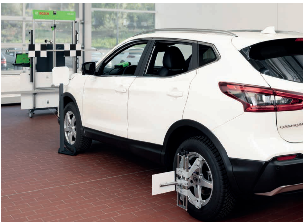
Nissan front radar + camera: The software based distance measurement shows it's full advantage especially at distances of 2-4 metres. That's a gain of workshop efficiency. Distance measurement aid with pointer for wheel centre reference.
