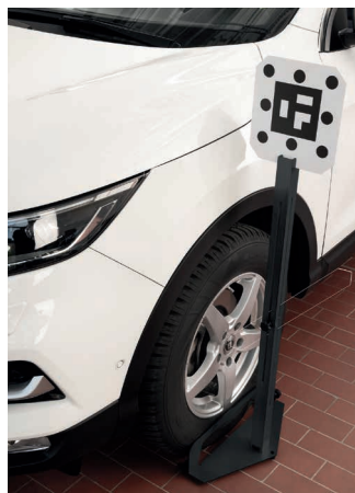
Nissan front radar + camera: The software based distance measurement shows it's full advantage especially at distances of 2-4 metres. That's a gain of workshop efficiency. Distance measurement aid with pointer for wheel centre reference.
