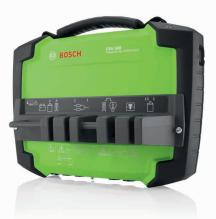
**FSA 500** The flexible entry point for simple diagnostics on electrical and electronic vehicle systems
