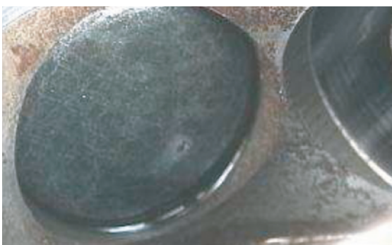
Corrosion at the high-pressure pump housing
