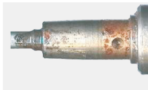
Corrosion at the injector
