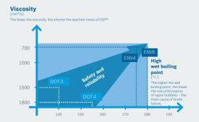
**ENV6 and ESP®:** Right from the development stage, modern brake fluids, such as Bosch ENV4 and ENV6 are designed to cope with the demands of current and future ESP® systems.
