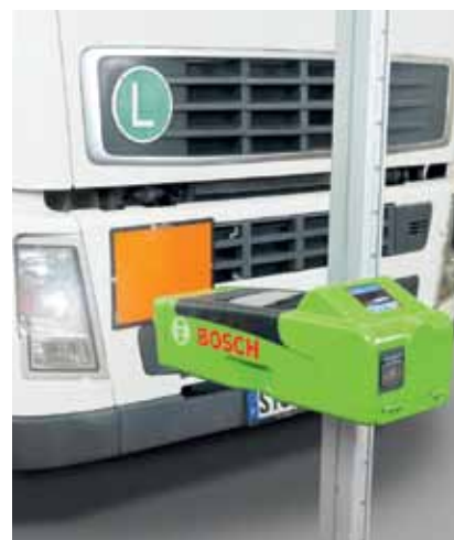
Bosch HTD 815: digital headlight tester
