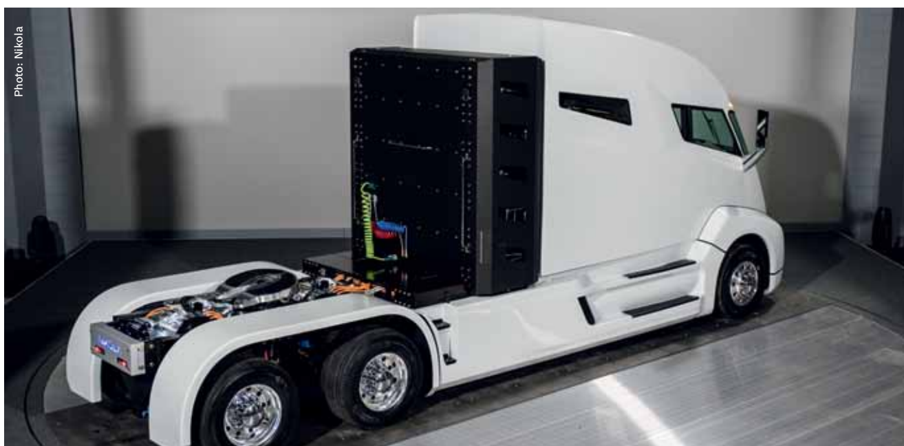
Bosch and Nikola electrify trucks with fuel cells and electric powertrains.
