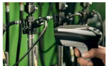
QualityScan: In order to identify the injector, the data matrix code can be read via scanner
