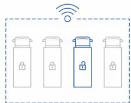
Sensors detect the digital key and unlock the vehicle doors.
