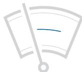
Max. 1 streak remains on the main field of view. Install a new wiper blade.
