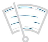
Max. 4-5 streaks remain on the outer field of view, or max. 12 streaks on the whole field of view. Install a new wiper blade.
