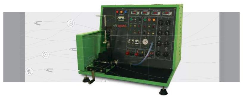
The new 3-Phase Auto Electrical Test Bench comes with advanced features to ensure the testing of even higher capacity Alternators from Bosch. This Test Bench is loaded with features that makes it extremely efficient and very safe to handle.
