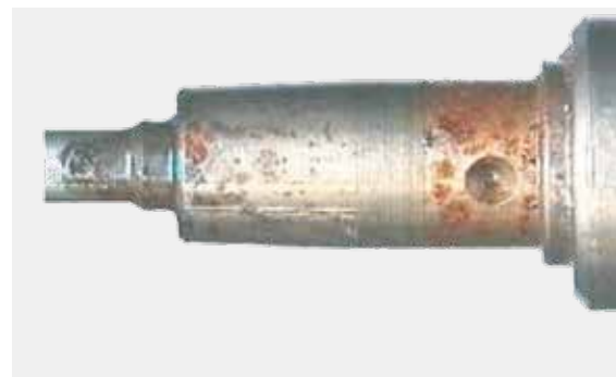
Corrosion at the injector
