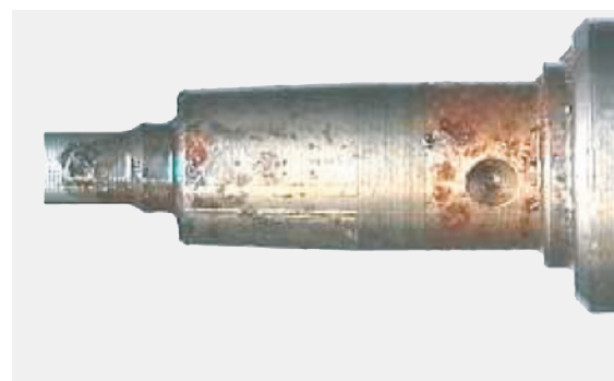
Corrosion at the injector
