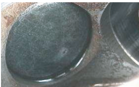
Corrosion at the high-pressure pump housing
