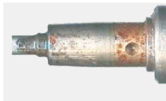
Corrosion at the injector
