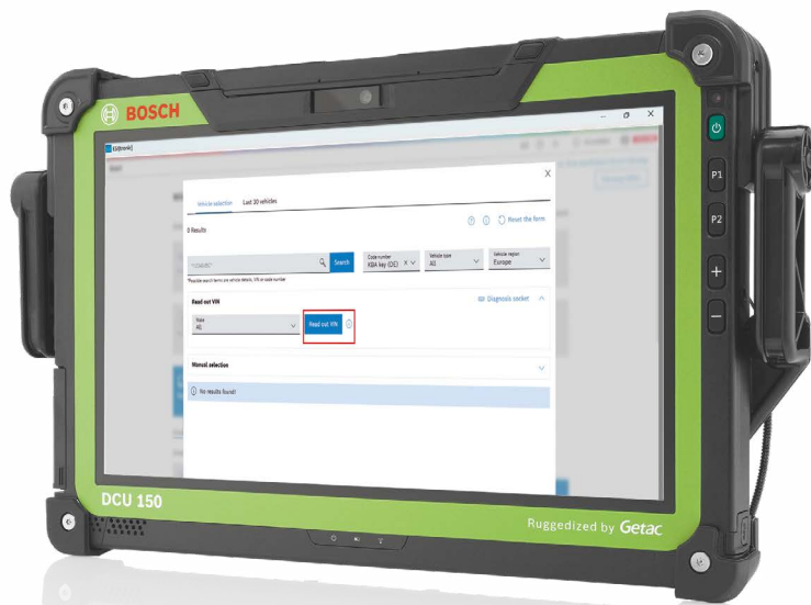
ESI[tronic] on DCU 150: fast vehicle identification with new direct search
