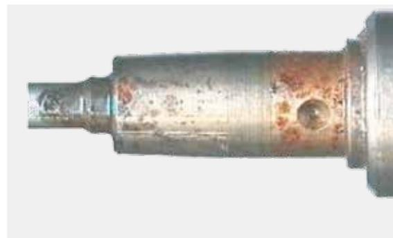
Corrosion at the injector
