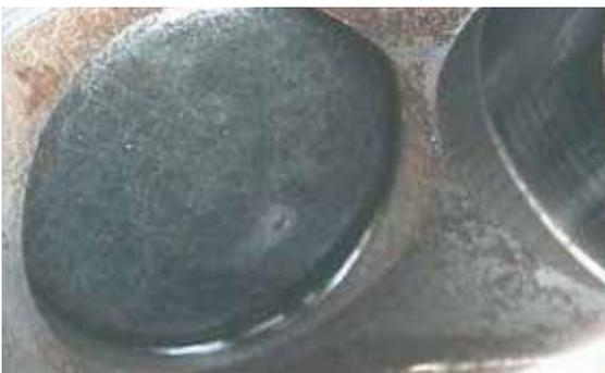
Corrosion at the high-pressure pump housing
