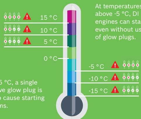
Below 5 °C, a single defective glow plug is likely to cause starting problems.
