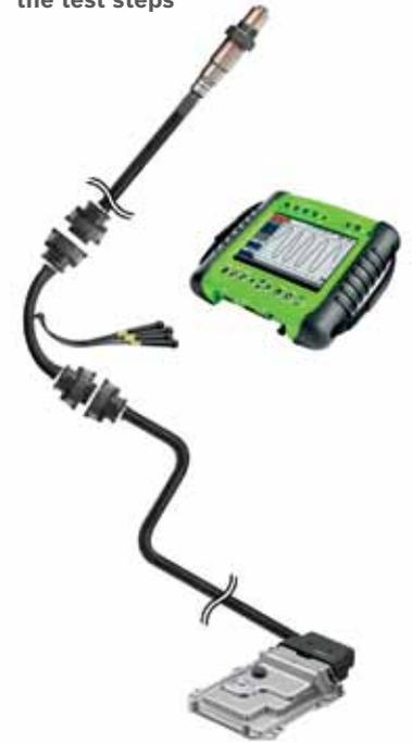
When analyzing the lambda sensor, please note the type of engine, the purpose of application (control or diagnostic sensor) and the operating conditions. Excess of air at the mixture formation can be a normal operating condition (diesel, fuel stratified direct injection, lean-combustion engines, ...)
