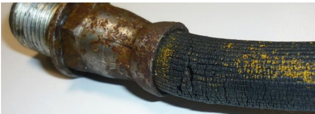
Corroded brake hose
