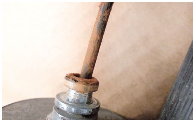
Corroded and tight brake cable
