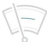
Max. 1 streak remains on the main field of view. Better install a new wiper blade.
