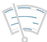
Max. 4-5 streaks remain on the outer field of view, or max. 12 streaks on the whole field of view. Better install a new wiper blade.
