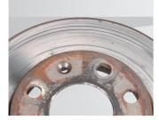
► Dirt particles on brake disc and pad
