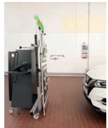
3-point radar calibration: Tilting positions according to OEM requirements: +2^\circ , 0^\circ , -2^\circ
