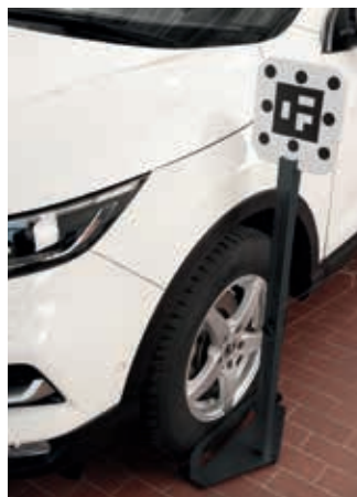
Nissan front radar + camera: The software based distance measurement shows it's full advantage especially at distances of 2-4 meter. That's a gain of workshop efficiency. Distance measurement aid with pointer for wheel centre reference.
