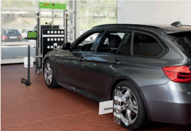
BMW/Mini and VW-Group: Highly precise placement towards the driving axis including specific distance setting. VW-Target installed vertical and centred in front of Radar sensor.
