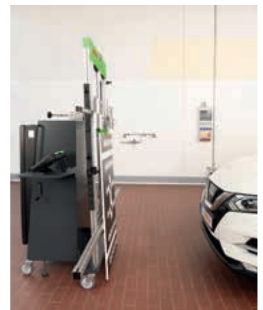
3-point radar calibration: Tilting positions according to OEM requirements: +2°, 0°, -2°
