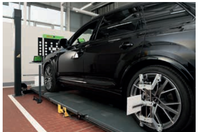
Above floor lifts: Program routine for permanent yaw angle display for monitoring if target is perpendicular to driving axis.
