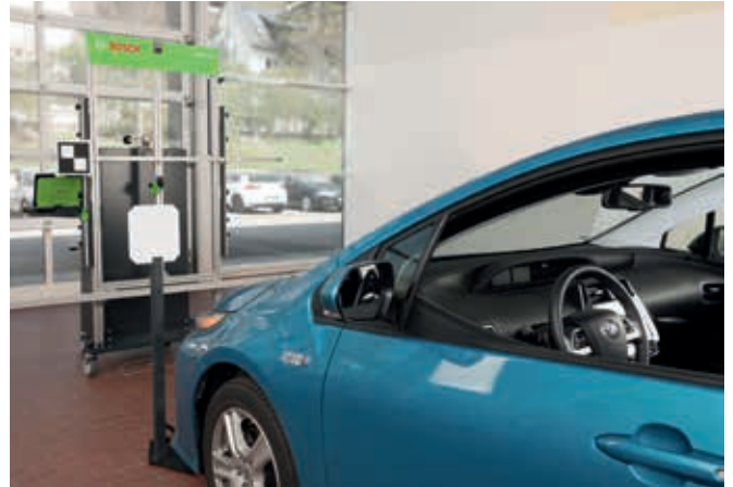
Toyota front camera: Sequential calibration with one or multiple targets. Highly precise positioning of the distance measurement aid according to OEM requirements.
