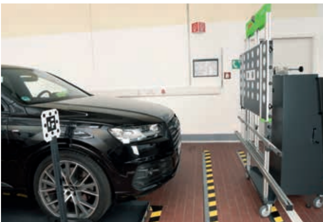
Headlight aimer bay: trouble-free placement between the rail systems. Ensured by large wheels, distance measurement aid and roll/pitch angel setting directly on the measurement bar.
