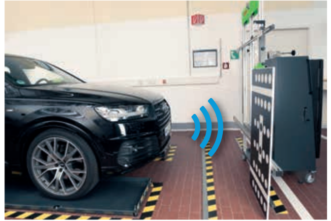
Audi: Double-Radar calibration with short setup time. Attach VW-Target to match with left and right radar axis. Lateral adjustment with a sense of proportion. Thanks to innovative product design, no height adjustment required.
