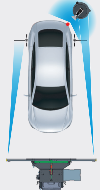
CTA 120 placement for corner radar with DAS 3000
