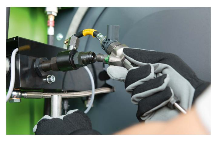
The latest exhaust emission standards and future directives increase the significance of testing common-rail injectors in modern diesel engines. Therefore, the more precise the measurement is, the more accurately the injector can be adapted.
