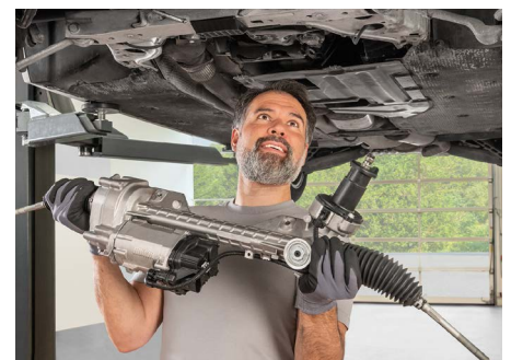
Steering installation in the workshop
