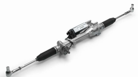
Bosch EPSapa with fail-operational function
