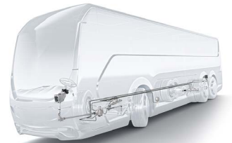
Commercial-vehicle steering system with rear axle steering
