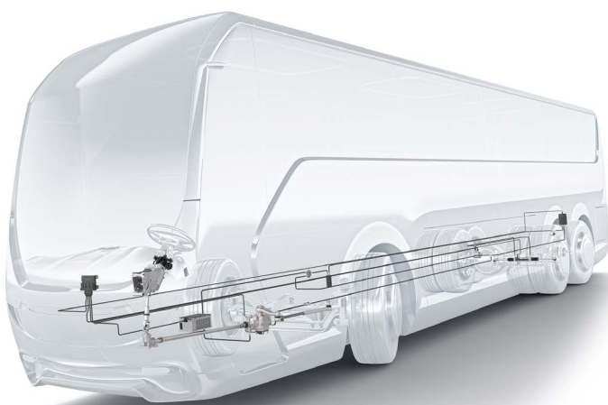
Commercial-vehicle steering system with rear-axle steering
