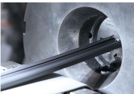
During extrusion, different rubber materials are blended to form the wiper lip and rubber back
