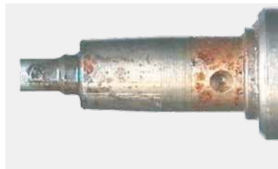
Corrosion at the injector
