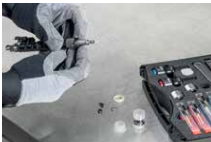
Assembly of the new decoupling element
