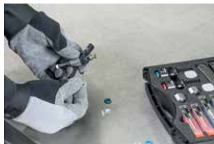
Disassembly of the O-ring and the support washer
