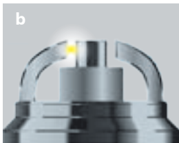
Side electrode – center electrode
