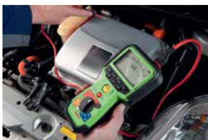
Voltage measurement via Bosch FSA 050
