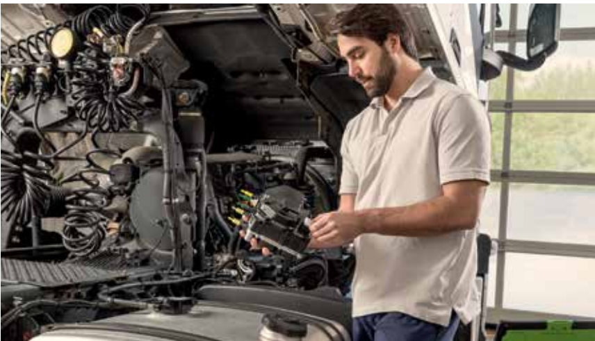
Replacing a Bosch supply module on a truck
