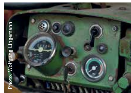
Fendt F225GT equipment carrier (1961–1965) with Bosch glow indicator, push button, rotary switch for the lights, pull switch and glow-plug starter switch
